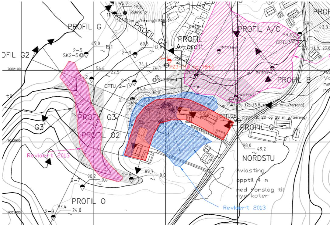
Figure 3 Plan view with a sketch over the area required (red) for soil improvement (existing houses not considered in this sketch).
