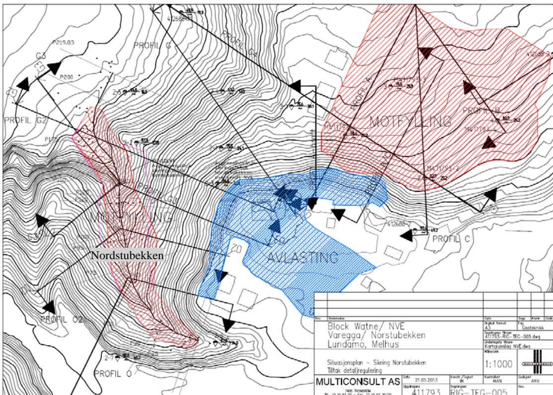
Figure 1 Plan view over the Lundamo slope and suggested measures with topographical changes. Drawing from Multiconsult (2013).
