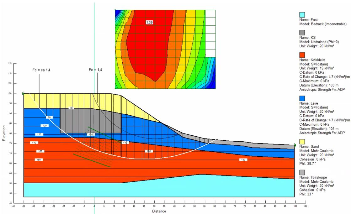
Figure 2 Result of a stability calculation with soil improvement (Profil A in Fig. 1).
